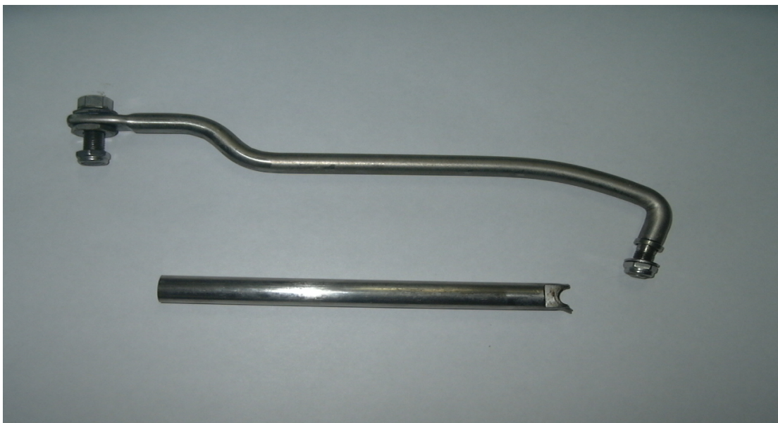
Photo 6 Failed drag link bar and hydraulic ram extension rod
