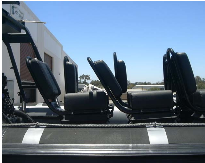
Photo 6 Seat damage resulting from RIB capsize
