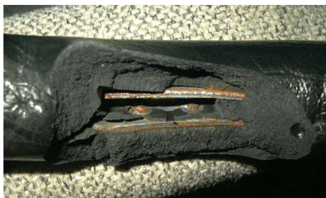
Photo 5 Helm wheel failed structural connection hidden by grip rubber
