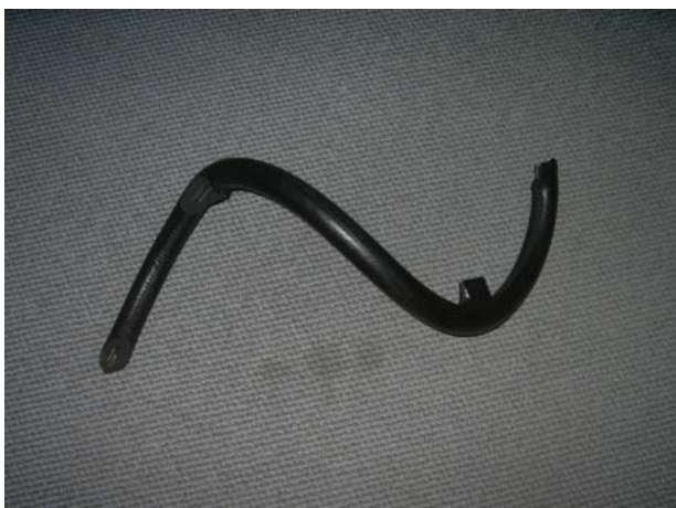
Photo 4 RIB helm wheel post accident
